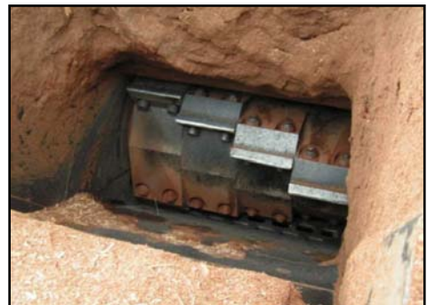
Looking down the throat of the hog inside the infeed chute of the wood chipper shows the hammers that pulverize wood into boiler fuel.
