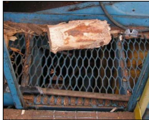
The 18-inch chunk of wood that struck the victim was only slightly shaved by the hog before it was forcefully ejected beyond the open hood of the bin.
