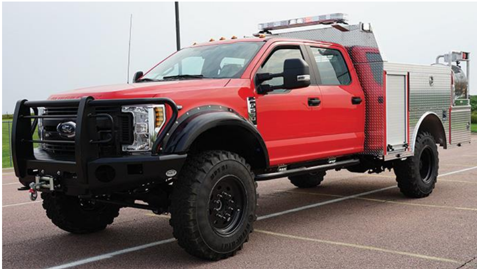
Image 1. Example of a Type 6 Wildland Fire Engine (Fire Apparatus & Emergency Equipment Staff, 2019).
